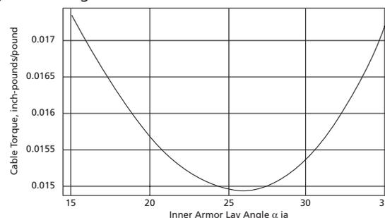
The actual computation of cable torque under load is a complicated problem as when the angles of inner and outer armor are changed, the tension carried by each layer and the torque are changing.
